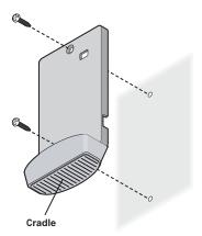
**2** Route the power and Ethernet cables through the large opening in the cradle. Figure 5 shows a cable being routed under the cradle.
